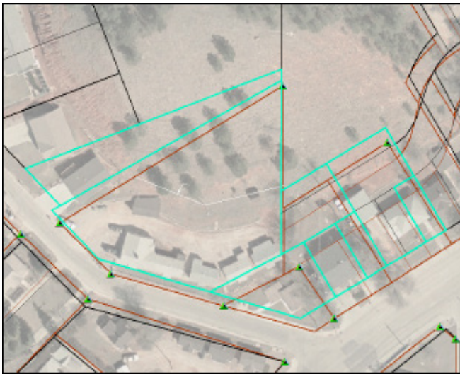
Figure 8. An example of an area of parcels that is well balanced geometrically with evenly distributed control
