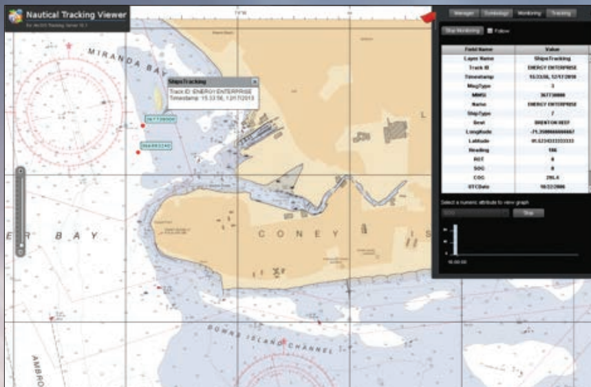
Figure 5: Integration of Electronic Navigational Chart with Live Vessel Tracking, off of Coney Island in New York City
