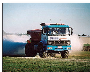
Ravensdown had already equipped a number of its fertilizer application trucks with GPS-controlled guidance systems and spreaders that captured location, fertilizer type, and spreading data.
