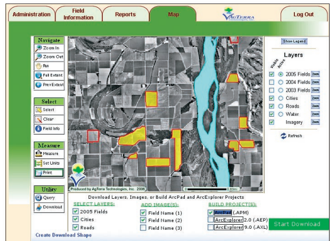
Based on ArcIMS, AgTerra's AgTrac application helps link tabular field data with spatial data to help direct field-based activities such as crop scouting, soil sampling, and ground-truthing remote imagery.
