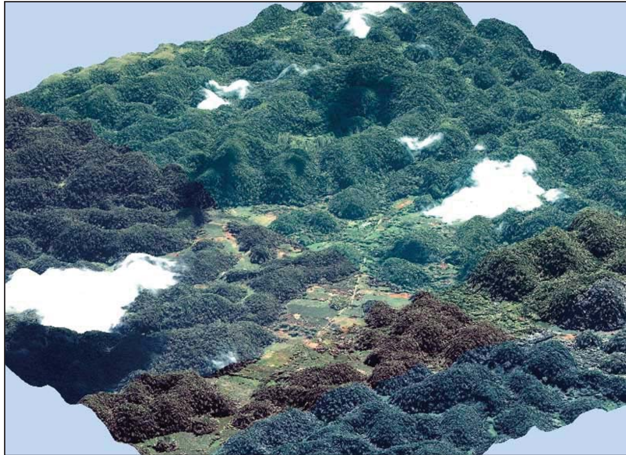
IKONOS satellite imagery of part of Cockpit Country was draped on a triangulated irregular network (TIN) representation of the terrain to provide photorealistic depictions of the study areas that were useful both before and after fieldwork.
