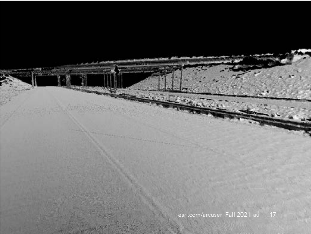
↓ Idaho interstate highway bridge, seen as a lidar depth surface in Street Smart.
