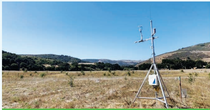
Eddy Covariance Tower —measuring carbon and water flux
