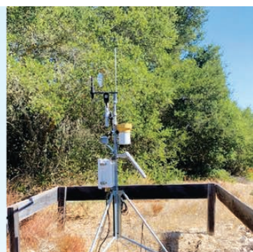
Weather Stations: temperature, RH, fPAR, wind, soil moisture
