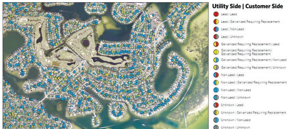
↑ Using the GeoAI toolbox in ArcGIS Pro enabled city staff to inventory drinking water assets.
