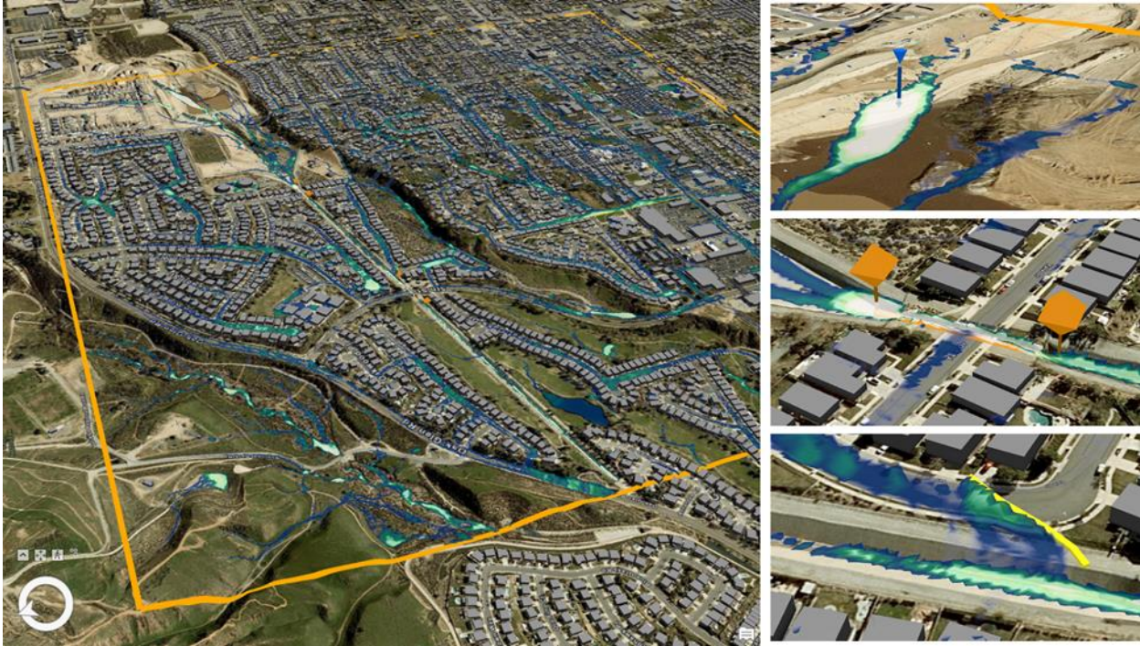
Figure 5. Rainfall simulation for an area of interest, with water source points, channels, and barriers
