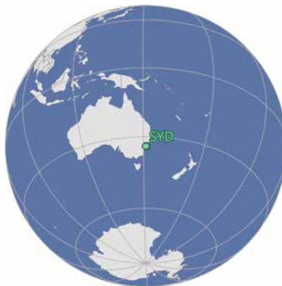
FIGURE 1.34. Orthographic projection centered on Sydney airport (SYD) with a grid which sketches spherical shape.
