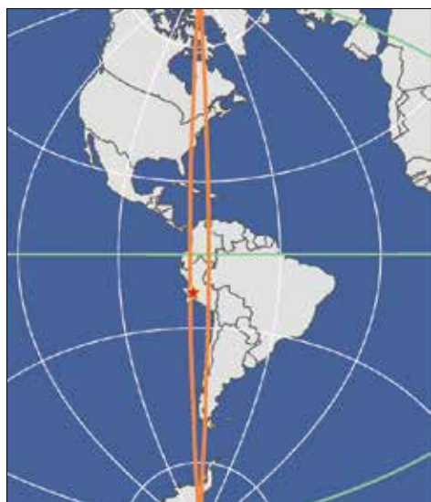
FIGURE 1.30. A pair of UTM zones outlined in orange: 18N and 18S. They span 72° to 84° west longitude and from 80° south to 84° north latitude. The entire map is projected using the zone 18 pair.
