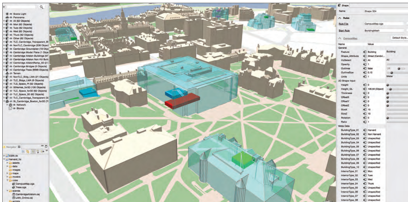
↑ After 3D models from CAD or photogrammetry are prepared, the data is imported and formatted using Esri CityEngine.
