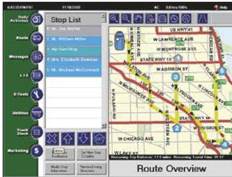
Mobile GIS application gives service technicians access to work order information such as schematic diagrams. The application also includes in-vehicle navigation capabilities and fleet mobile mapping and routing modules. This has increased technicians' productivity by 10 percent daily.
