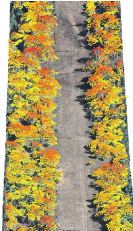
Tree height values are displayed as points created from the same digital aerial imagery. ArcGIS 3D Analyst is used to identify tree canopies that put the network at risk.
