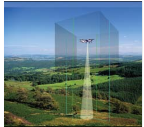
A gas detection and measuring sensor is integrated into aircraft that fly over right-of-way corridors.
